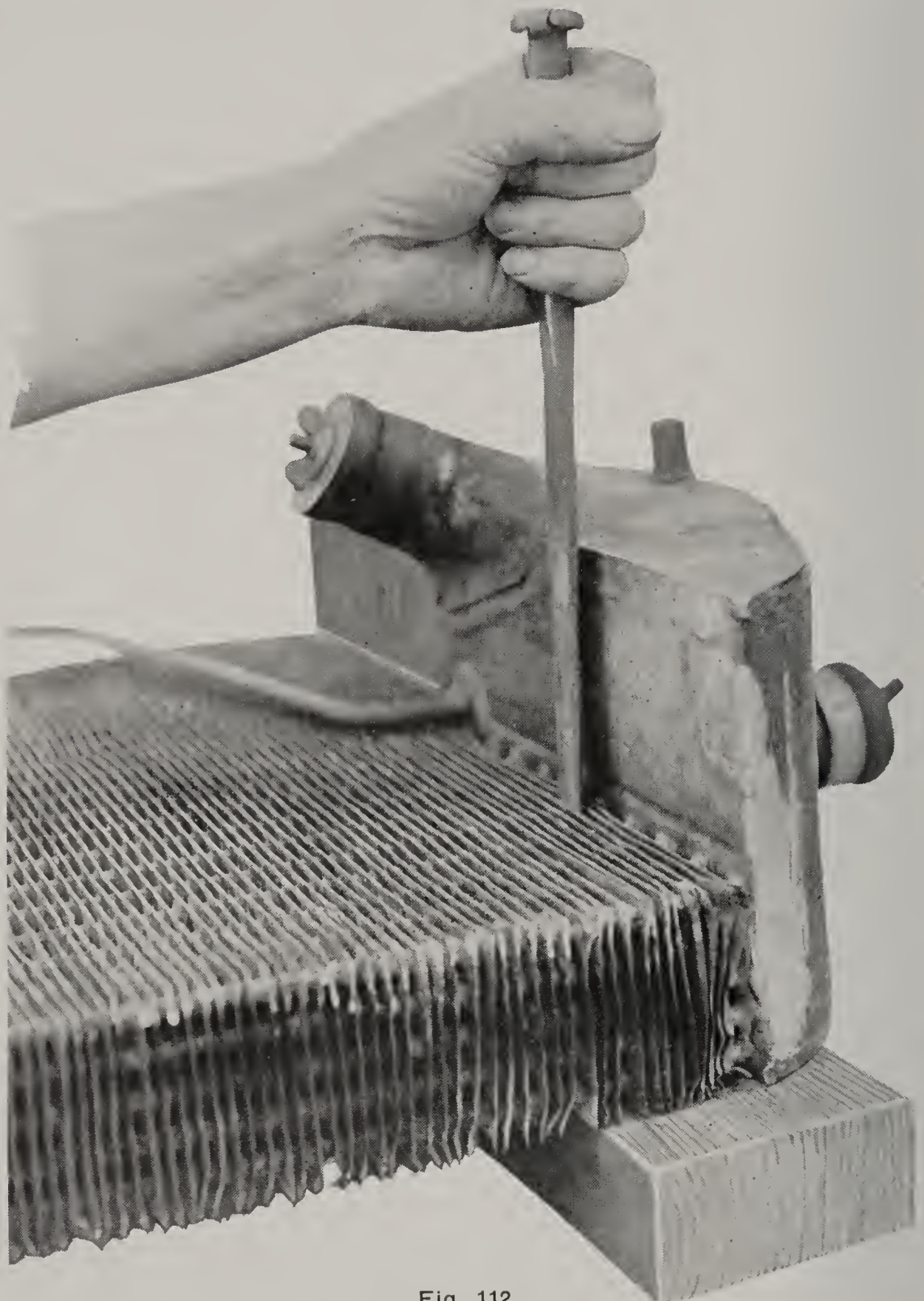
Fig. 112 Cutting Tank From Damaged Core
